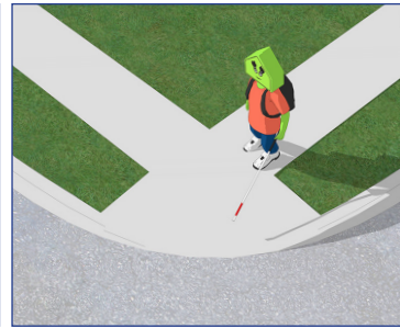
Missing tactile pavers
