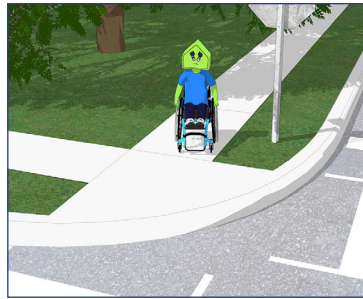
Missing curb ramps
